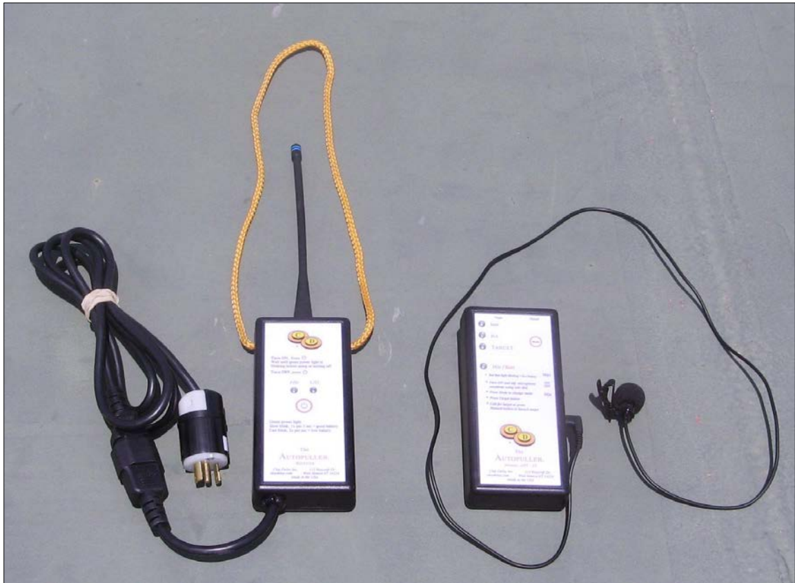
Figure-1: Auto-puller Receiver Unit with yellow cord (left), and Auto-puller Controller Unit with microphone (right).
